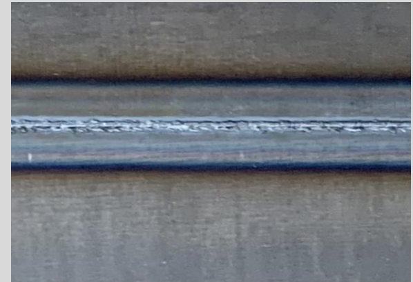
Blech: S355, 6 mm (Unterseite)
